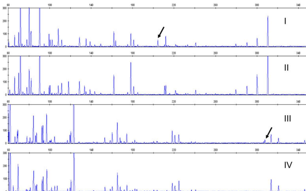
**Figure 4.** AFLP electropherograms illustrating polymorphism between bulked DNA samples of wild mustard NILs. Panels I and III show specific peaks representing markers 2 and 5 (arrow), respectively, present in resistant and absent (panels II and IV) in susceptible samples.
