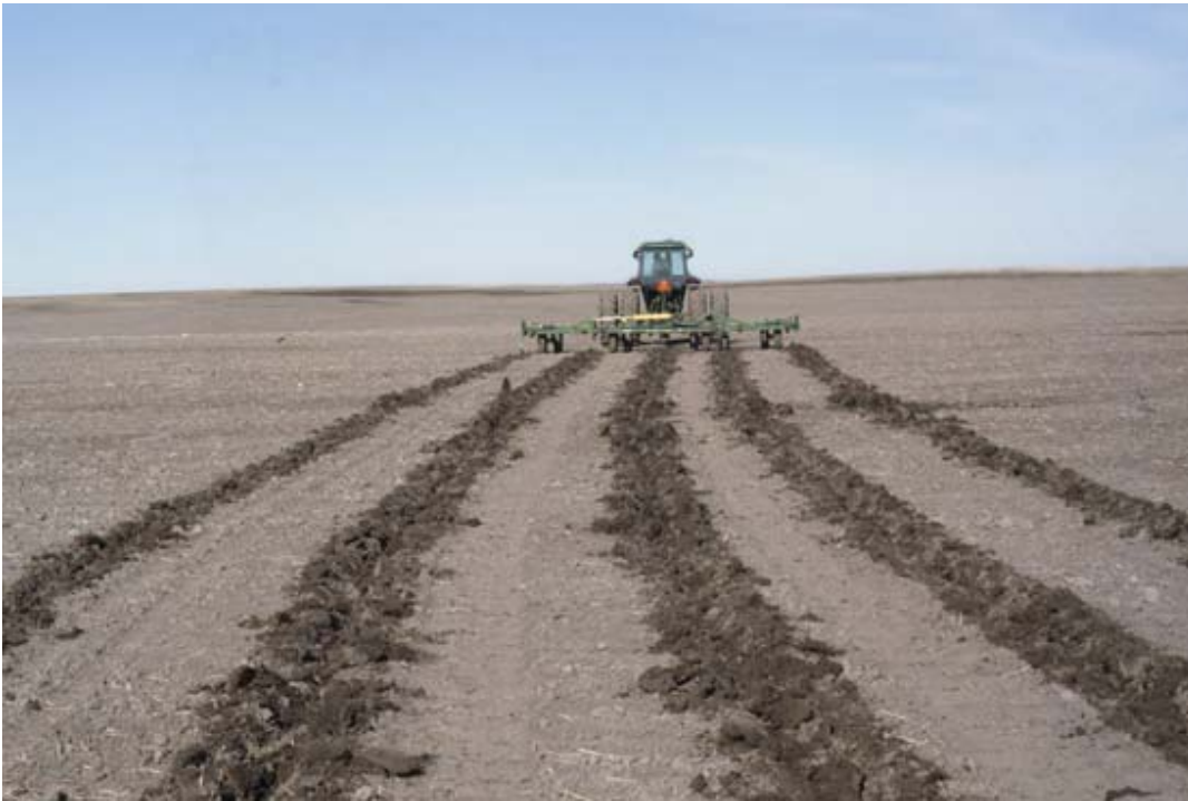
Widely spaced shanks used for emergency tillage, making clods to roughen the soil surface. Photo courtesy of University of Nebraska.
