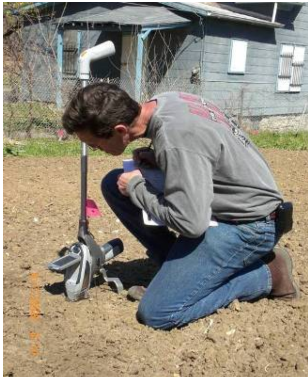
Blasé Leven, K-State's Center for Hazardous Substance Research, doing preliminary in situ soil screening at the Kansas City site using handheld X-ray fluorescence.
