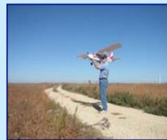
Large high-wing trainer aircraft, such as the Super Frontier Senior from World Models, make excellent UAVs. This plane has an 2.05 m wingspan and weighs 5.7 kg when fully loaded. Takeoffs and landings are difficult because runways and landing zones are not available at most research sites. The aircraft is hand launched and landed with no power (deadstick). It often comes to an abrupt stop in tall grass or weeds. A folding propeller is used to avoid damage on impact.
