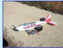
The UAV is powered by a MaxCim 13Y brushless motor running on 20 Sanyo 2600 mA Nimh batteries (the batteries can be seen protruding through the firewall under the motor). When driving a 14x10 folding propeller on a 3.33:1 gearbox, over 1000 W of power are generated (see ElectricCalc analysis).
