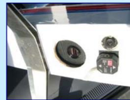
The underside of the UAV showing the camera bay opening, the down-facing video camera, and the FMA co-pilot sensor. When activated, the co-pilot module uses infrared transducers to keep the plane flying straight and level ([www.fmadirect.com](http://www.fmadirect.com)).
