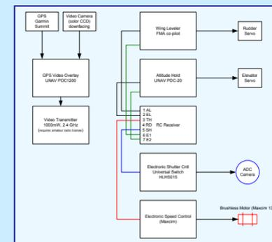
Block diagram of the avionics used in the UAV.
